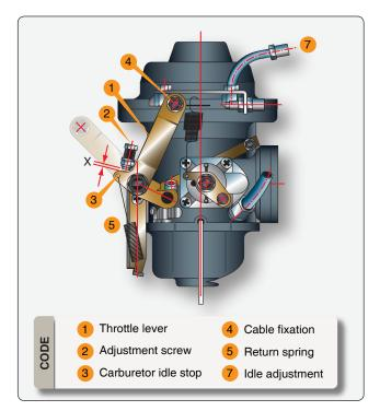
Figure 11-27. *Carburetor throttle lever*.
