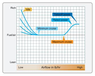
Figure 10-48. Idle mixture curve.
