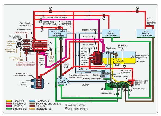
Figure 6-46. Typical turbine dry-sump variable pressure lubrication system.
