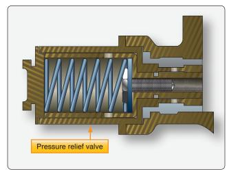
Figure 6-38. Pressure relief valve.
