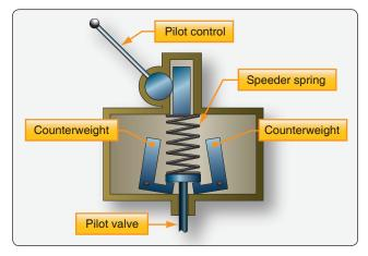
Figure 7-17. Underspeed condition.
