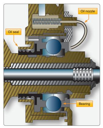
Figure 6-39. Oil nozzles spray lubricate on bearings.
