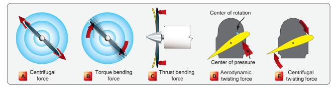
Figure 7-8. Forces acting on a rotating propeller.
