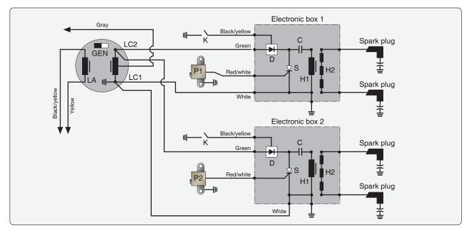
Figure 11-5 Rotax 503 and 582 electrical system.
