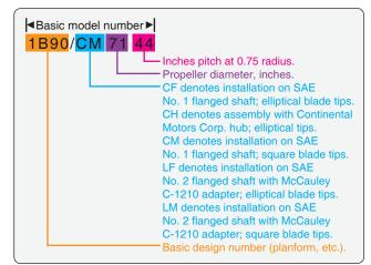
Figure 7-23. Complete propeller model numbers.
