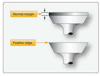
**Figure 10-26.** *Engine valves showing normal margin and a feather edge.*
