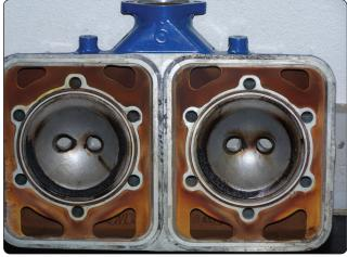
Figure 11-8. Water-cooled heads.
