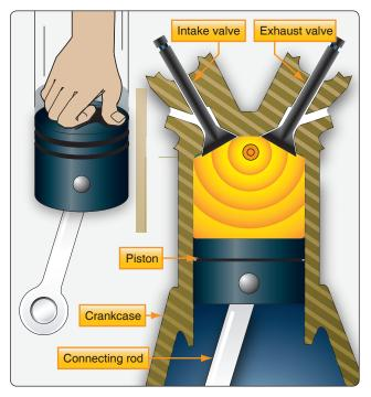
Figure 10-42. Normal combustion within a cylinder.
