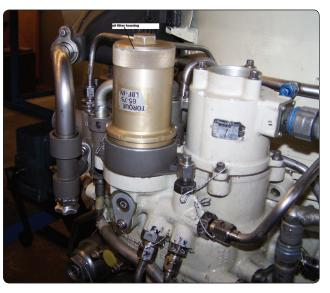
Figure 6-48. Oil filter housing.
