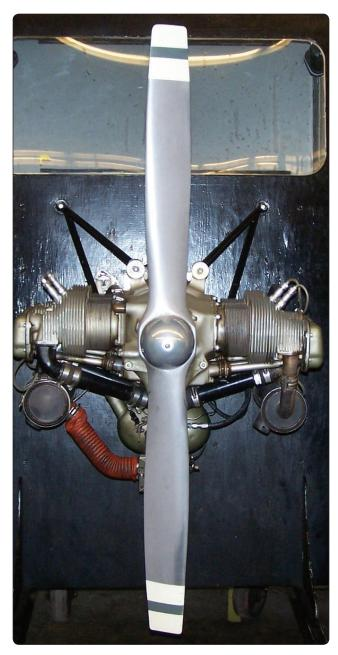
Figure 7-11. Fixed-pitch propeller.
