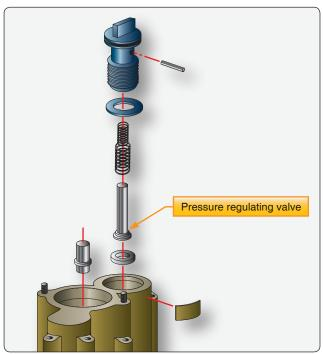
Figure 6-37. Pressure regulating valve.
