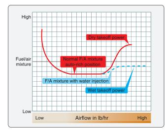
Figure 10-46. Fuel/air curve for a water-injection engine.
