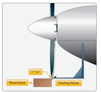
Figure 7-34. Propeller blade tracking.
