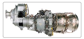
Figure 7-45. Pratt & Whitney 150 turboprop engine.
