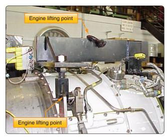
Figure 8-9. Hoisting sling attached to engine.
