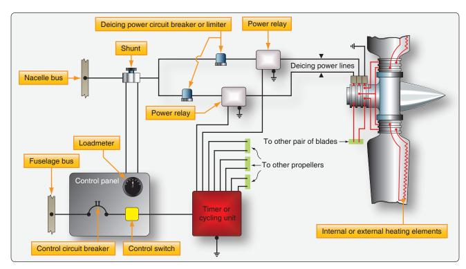
Figure 7-28. Typical electrical deicing system.
