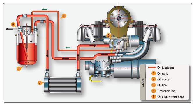
Figure 11-10. Lubrication system.
