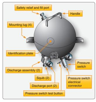
Figure 9-23. Fire extinguishing bottle.
