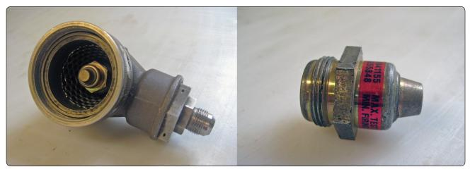
Figure 9-10. Discharge valve (left) and cartridge (squib) (right).
