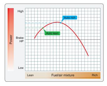
Figure 10-44. Power versus fuel/air mixture curve.
