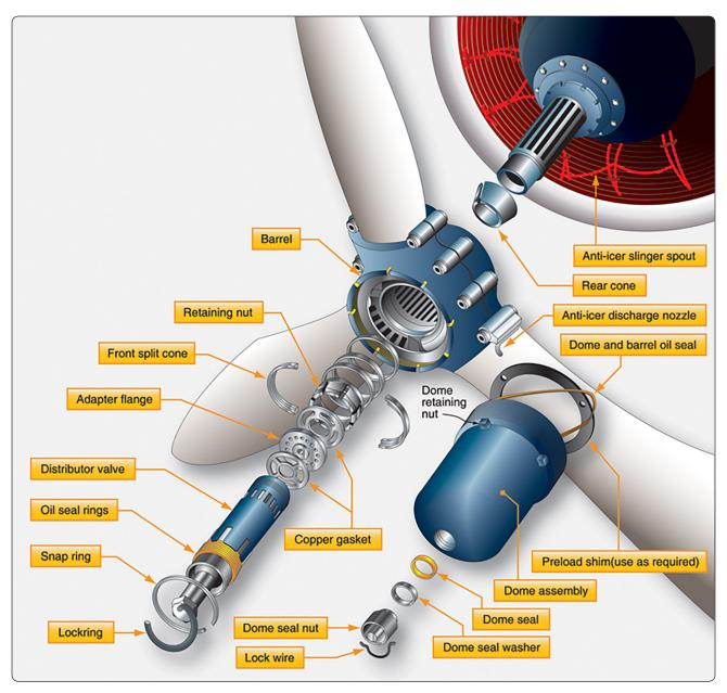
Figure 7-55. Typical hydromatic propeller installation.
