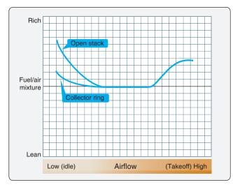
**Figure 10-50.** *Comparison of fuel/air mixture curves for open-stack and collector-ring installations.*
