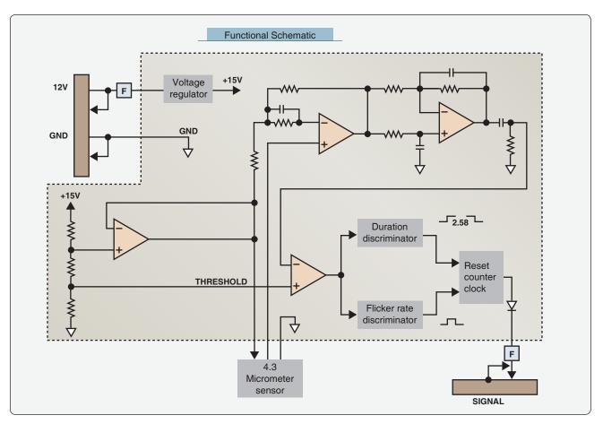
Figure 9-3. Optical fire detection system circuit.
