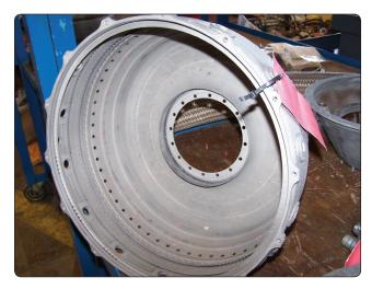
Figure 10-63. Combustion case inspection.
