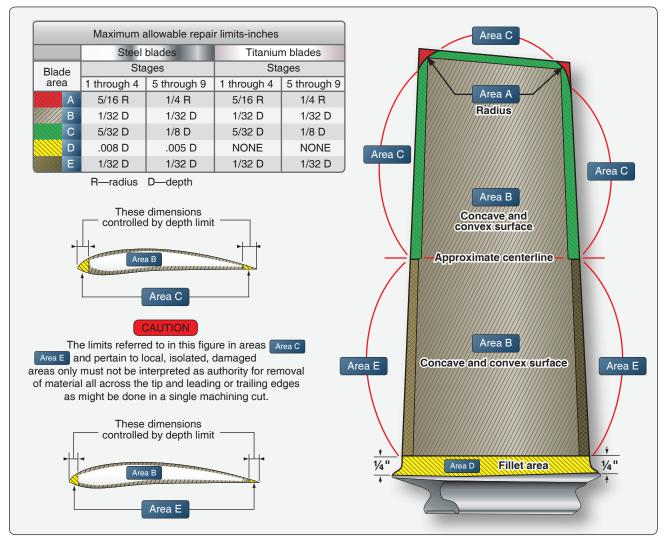
Figure 10-57. Typical compressor blade repair limits.
