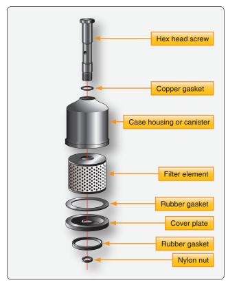
Figure 6-7. Housing filter element type oil filter.
