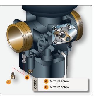
Figure 11-28. Idle mixture screw.
