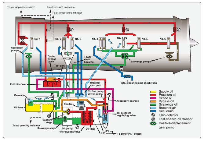
Figure 6-45. Typical turbine dry-sump pressure regulated lubrication system.
