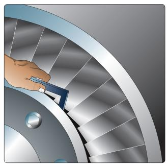
Figure 10-71. Measuring turbine wheel to exhaust cone clearance.
