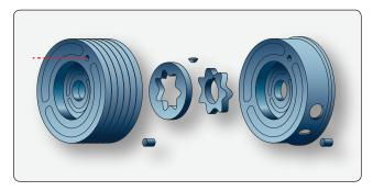
Figure 6-33. Typical gerotor pumping elements.
