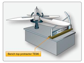
Figure 7-36. Bench top protractor.
