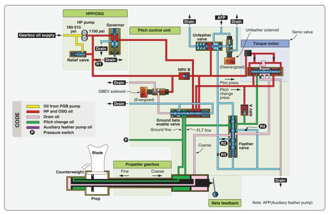
Figure 7-48. Propeller control system schematic.
