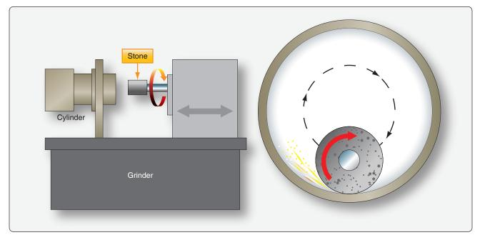
Figure 10-30. Cylinder bore grinding.
