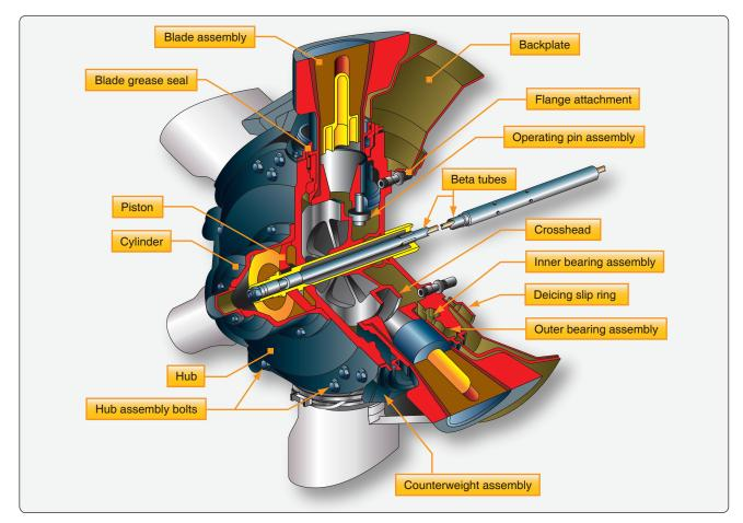
Figure 7-47. Turboprop propeller.
