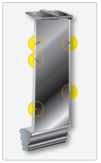
Figure 10-64. Stress rupture cracks.
