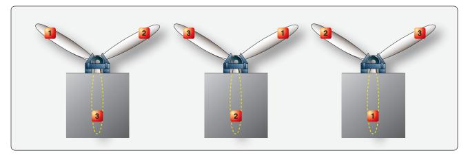
Figure 7-39. Positions of three-bladed propeller during balance check.
