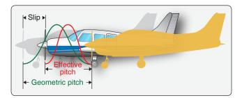
Figure 7-4. Effective pitch and geometric pitch.
