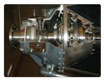
Figure 7-46. Reduction gearbox.
