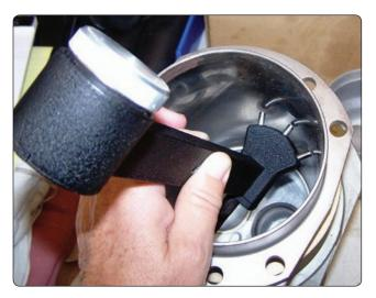
Figure 10-5. A cylinder bore gauge.
