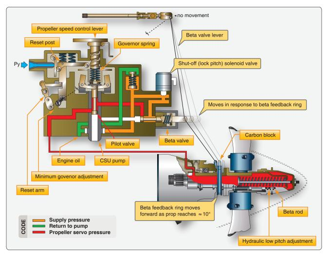
Figure 7-51. Beta mode forward operation.
