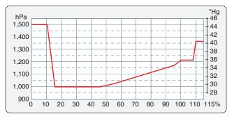
**Figure 11-13.** *Correlation between throttle position and nominal boost pressure.*
