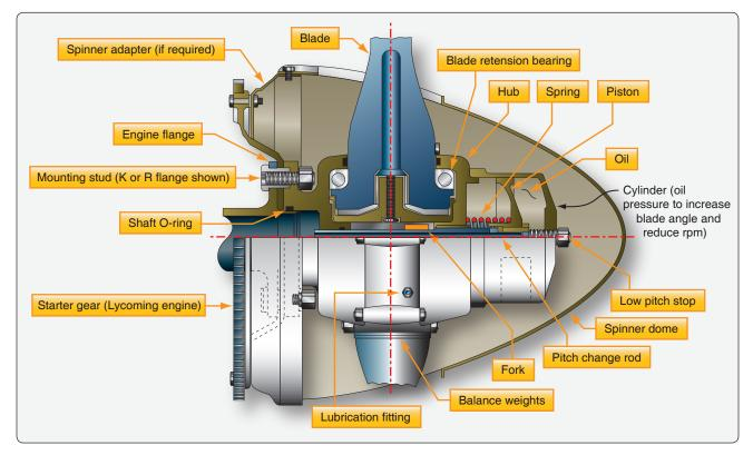
Figure 7-24. Constant speed non-feathering propeller.
