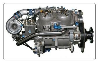
Figure 6-49. Diesel liquid-cooled aircraft engine.
