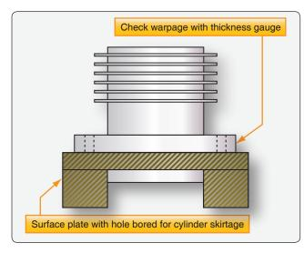
Figure 10-2. A method for checking cylinder flange warpage.
