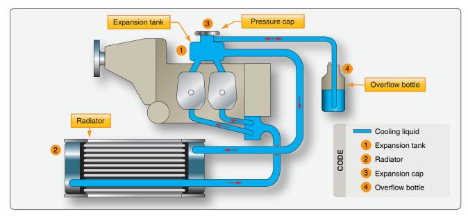
Figure 11-7. Rotax 914 cooling system.
