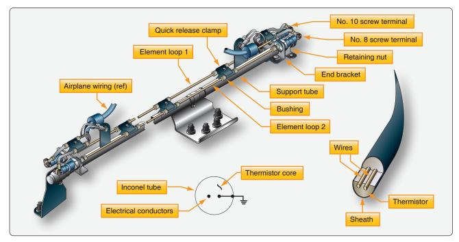
Figure 9-5. Kidde continuous-loop system.
