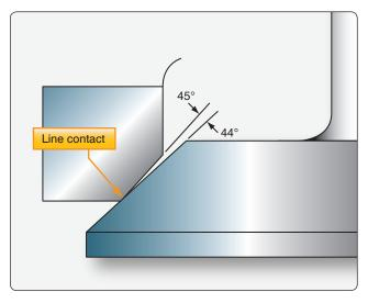
Figure 10-23. Interference fit of valve and valve seat.
