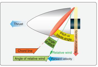
Figure 7-5. Propeller aerodynamic factors.
