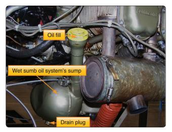
Figure 6-16. Basic wet-sump oil system.
