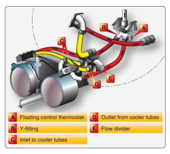
Figure 6-14. Dual oil cooler system.
