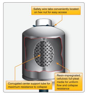
Figure 6-9. Cutaway view of a filter.
