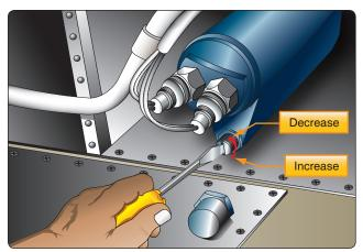
Figure 6-27. Oil pressure relief valve adjustment.
