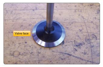
Figure 10-15. Valve face surface.
