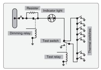
Figure 9-1. Thermal switch fire circuit.
