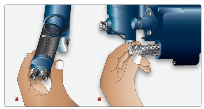
Figure 6-26. Oil pressure screen (A) and scavenge oil screen assembly (B).
