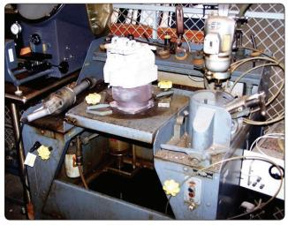
Figure 10-16. Valve seat grinding equipment.
