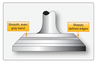
Figure 10-28. A correctly lapped valve.
