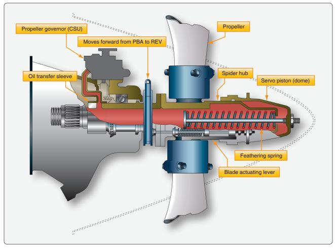
Figure 7-49. Pitch change mechanism.
