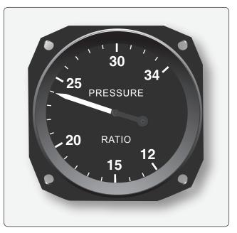
Figure 10-72. Engine pressure ratio indications.
