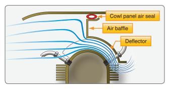
Figure 6-57. Cylinder head baffle and deflector system.
