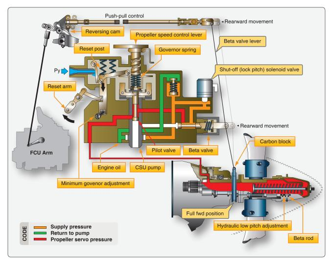
Figure 7-52. Beta mode reverse operation.
