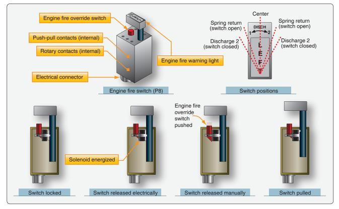
Figure 9-13. Engine fire switch operation.
