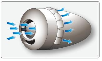
Figure 6-51. Regulating the cooling airflow.
