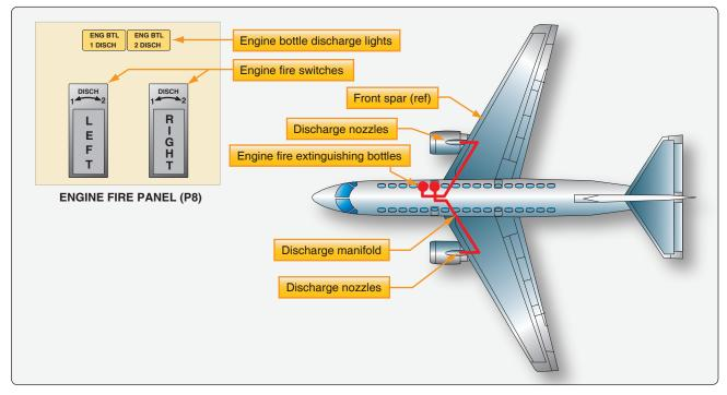
Figure 9-22. Boeing 777 fire extinguisher container location.
