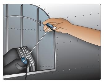
Figure 6-23. Checking oil level with dipstick.
