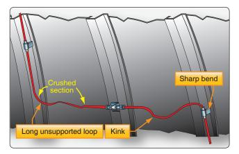
Figure 9-14. Sensing element defects.
