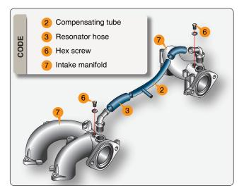
Figure 11-26. Resonator hose and compensating tube.
