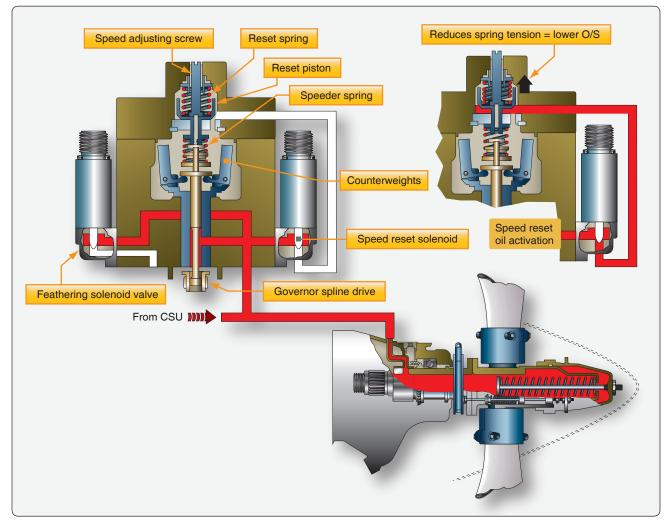
Figure 7-54. Propeller overspeed governor.
