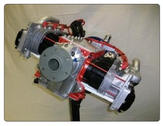
Figure 11-18. Aeromax direct drive, air-cooled, six-cylinder engine.
