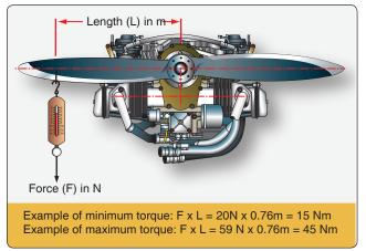
Figure 11-34. Checking propeller gearbox.
