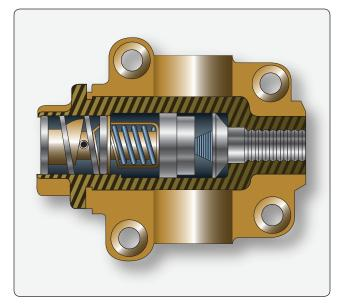
Figure 6-41. Typical thermostatic bypass valve.
