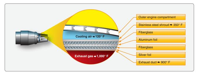
Figure 6-62. *Typical engine insulation blanket*.
