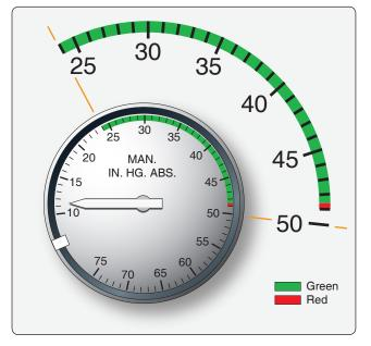
Figure 10-37. Manifold pressure gauge.
