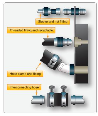
Figure 8-8. Types of line disconnects.
