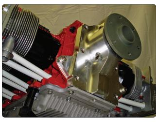
Figure 11-19. Front-end bearing on the 1000 IFB engine.
