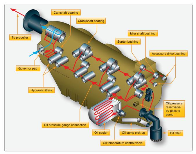
Figure 6-15. Oil circulation through the engine.
