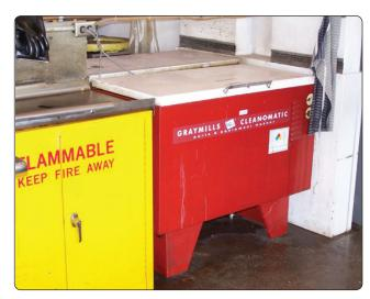
Figure 10-3. *Typical solvent degreasing tank.*
