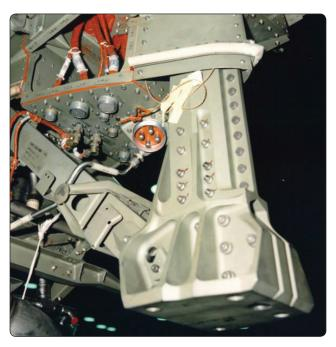
Figure 8-17. *Turbine engine front mount.*
