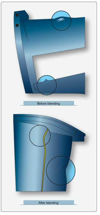
Figure 10-62. Guide vane trailing edge damage.
