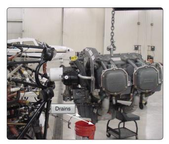
Figure 8-4. Oil system drain points.
