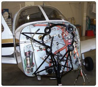
Figure 8-2. Typical firewall with components mounted on it.
