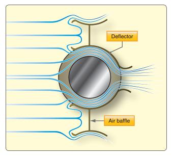
Figure 6-50. Cylinder baffle and deflector system.
