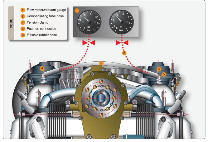
Figure 11-29. Gauges attached to the engine.
