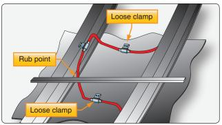
Figure 9-16. Rubbing interference.
