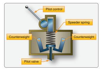
Figure 7-18. Overspeed condition.
