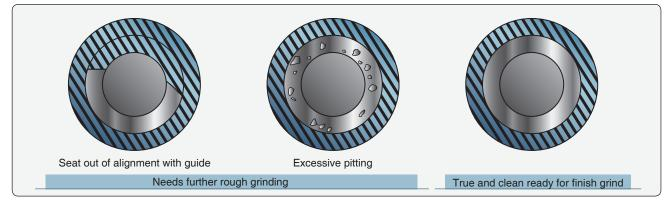
Figure 10-18. Valve seat grinding.
