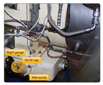
Figure 6-47. *Typical turbine wet sump system*.
