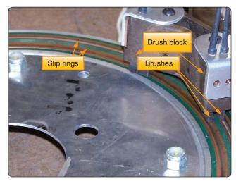
Figure 7-29. Deicing brush block and slip ring assembly.
