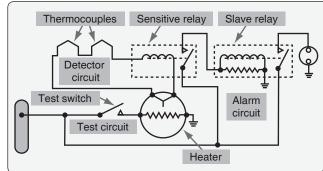
Figure 9-2. Thermocouple fire warning circuit.
