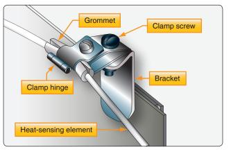
Figure 9-17. Inspection of fire detector loop clamp.
