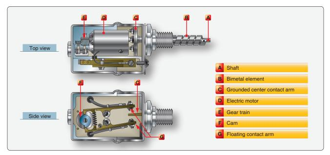
Figure 6-13. Floating control thermostat.
