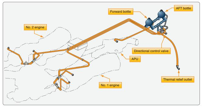
Figure 9-8. Typical fire extinguishing system.
