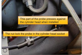
Figure 6-58. Bayonet type CHT probe.
