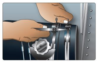
Figure 6-21. Removal of securing straps.
