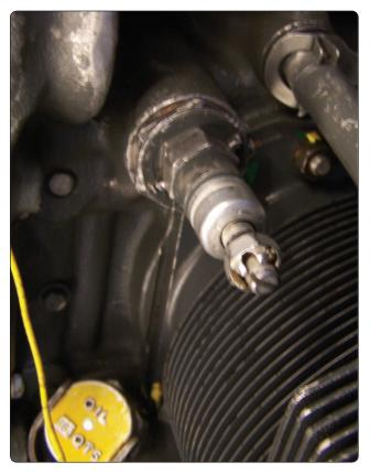
Figure 6-10. Oil pressure adjustment screw.
