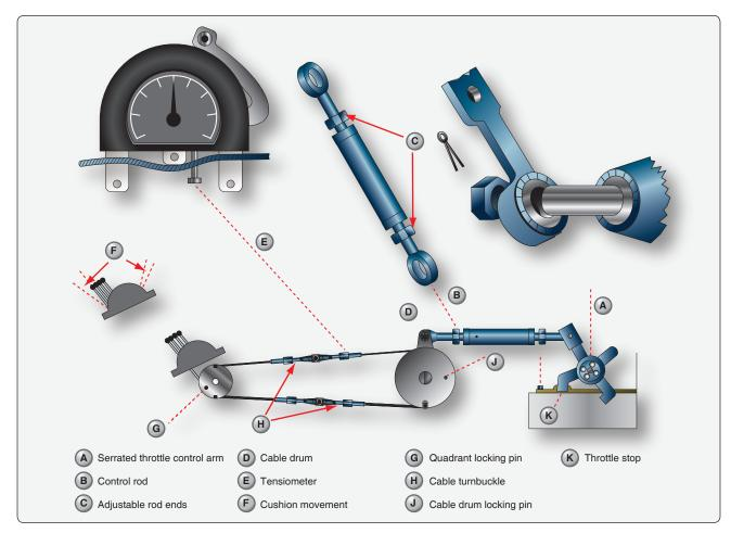
Figure 8-11. Schematic drawing of throttle control system.
