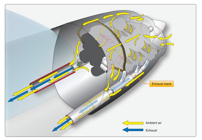
Figure 6-53. Engine cooling and exhaust system.
