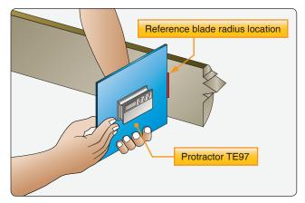
Figure 7-35. Blade angle measurement.
