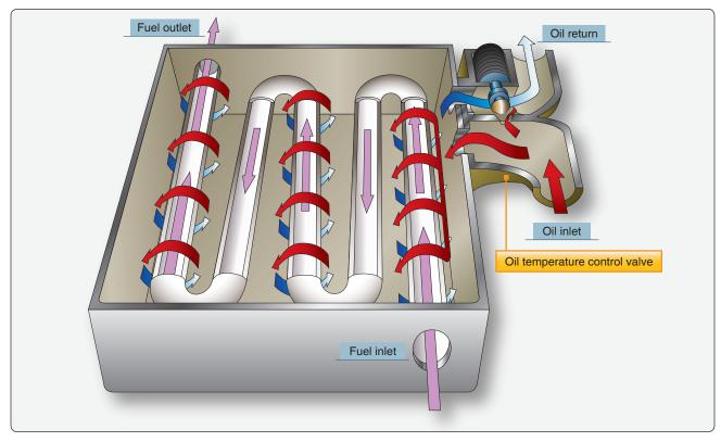
Figure 6-43. Fuel oil heat exchanger cooler.
