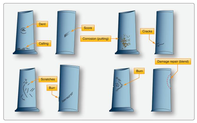
Figure 10-60. Compressor blade damage.
