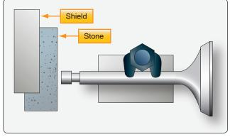
Figure 10-27. *Grinding a valve tip.*
