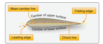
Figure 7-7. Cross-section of a propeller blade.
