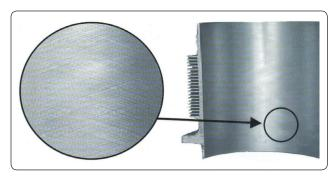
Figure 10-32. Cross-hatch pattern on cylinder wall.
