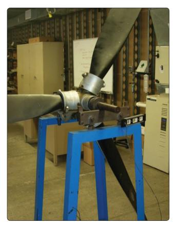
Figure 7-40. Static propeller balancing.
