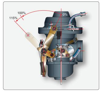
**Figure 11-12.** *Turbocharger control system throttle range and position.*
