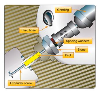
Figure 10-17. Valve seat grinding setup.
