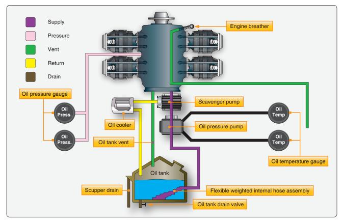
Figure 6-4. Oil system schematic.
