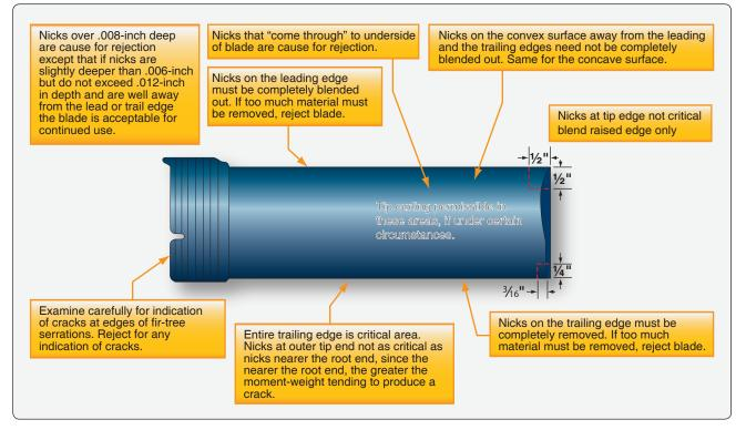
Figure 10-66. *Typical turbine blade inspection*.
