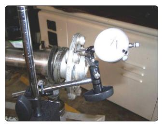
Figure 10-10. Checking crankshaft runout.
