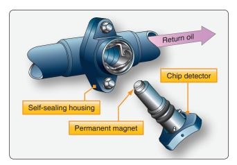
Figure 6-44. Chip detector.
