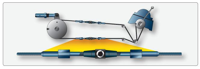
Figure 8-6. Engine control cable and turnbuckle assembly.
