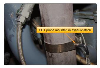
Figure 6-60. EGT probe in exhaust stack.
