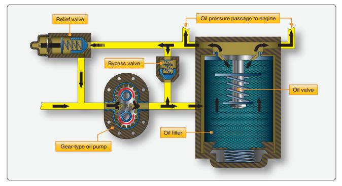
Figure 6-6. Engine oil pump and associated units.
