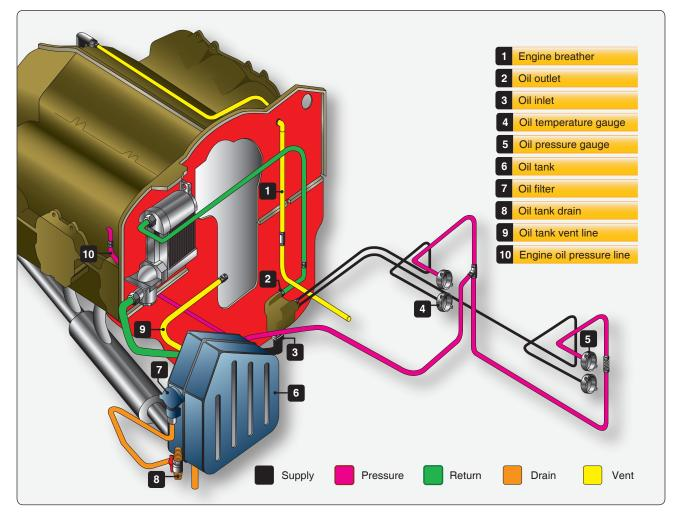
Figure 6-18. Oil system perspective.
