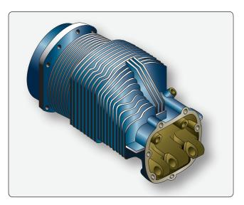
Figure 6-56. A cylinder head and fins.
