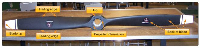
Figure 7-1. Basic nomenclature of propellers.
