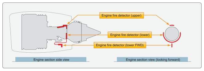
Figure 9-7. Large turbofan engine fire zones.
