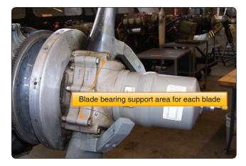
Figure 7-13. Blade bearing areas in hub.
