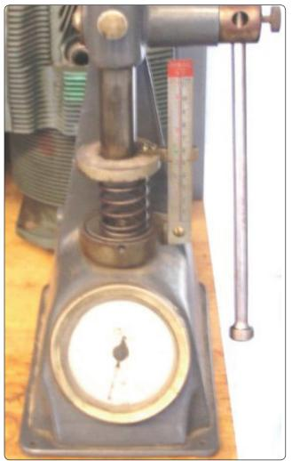
Figure 10-9. Valve spring compression tester.
