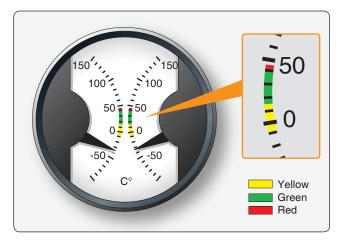
Figure 10-35. Carburetor air temperature gauge.
