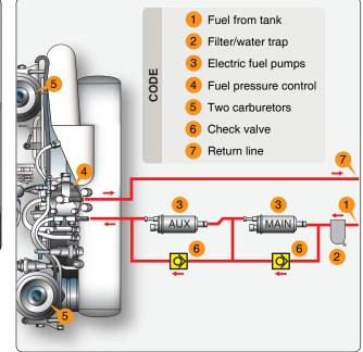
Figure 11-9. Fuel system components.
