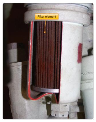
Figure 6-35. *Turbine oil filter paper element.*
