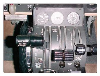
Figure 7-10. *Turboprop propeller controls*.
