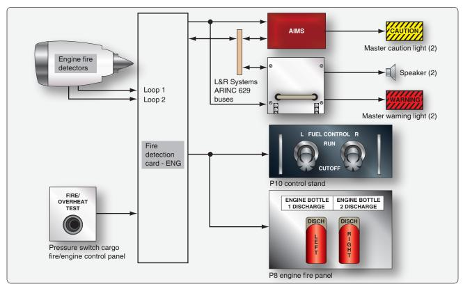
Figure 9-20. Engine fire detection system.
