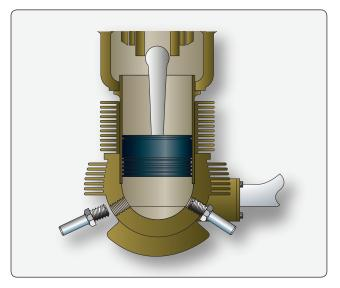
Figure 8-3. Draining corrosion preventive compound.
