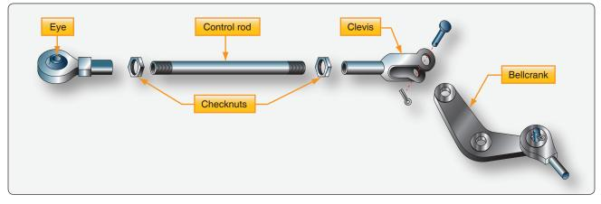
Figure 8-7. Engine control linkage assembly.
