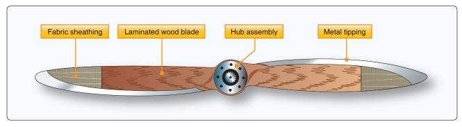
Figure 7-20. Fix-pitch wooden propeller assembly.
