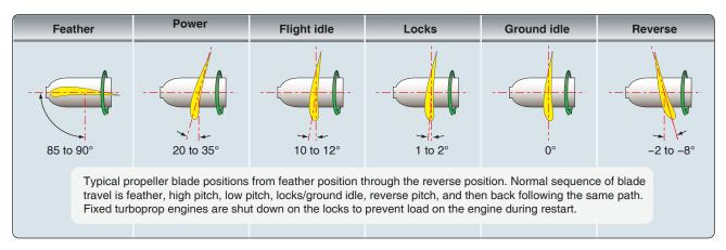
Figure 7-3. Propeller range positions.
