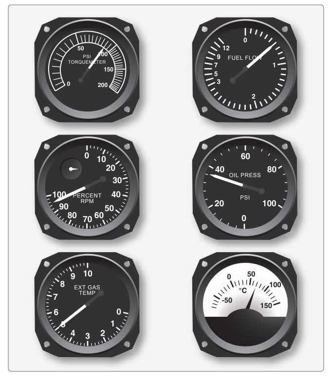
Figure 10-73. *Typical turbine engine instruments*.
