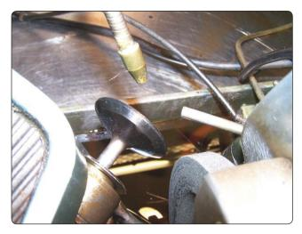
Figure 10-25. Valve in chuck ready to grind.
