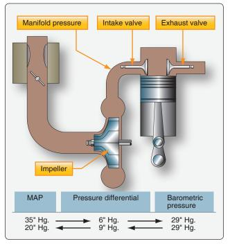
Figure 10-49. Effect of valve overlap.
