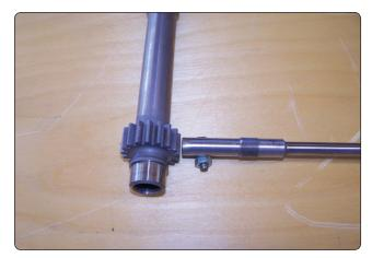
Figure 10-79. Magnetic pickup and gear.
