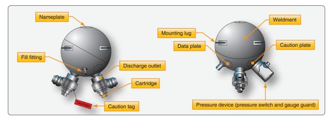
Figure 9-9. Fire extinguisher containers (HRD bottles).
