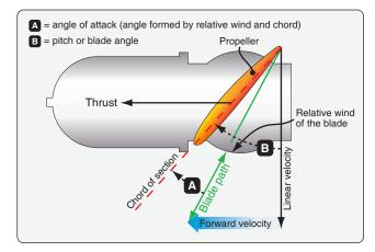
Figure 7-9. Propeller forces.
