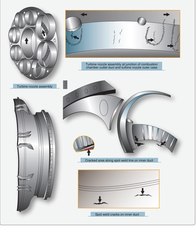
Figure 10-69. *Turbine nozzle assembly defects*.
