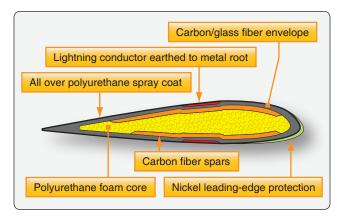
Figure 7-32. Composite blade construction
