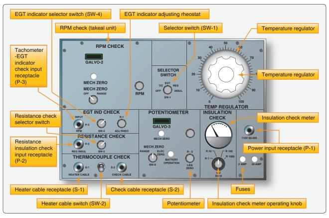
Figure 10-77. Jetcal analyzer instrument compartment.
