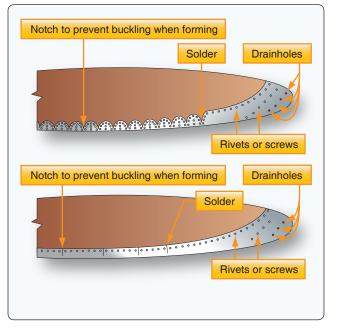
Figure 7-21. Installation of metal sheath and tipping.
