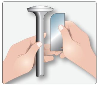
Figure 10-8. Checking valve stretch with a manufacturer's gauge.
