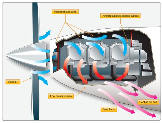
Figure 6-55. *Differential air cooling*.
