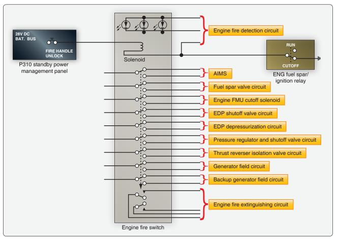
Figure 9-27. Engine fire switch circuit.
