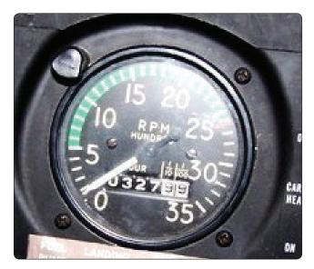
Figure 10-38. Tachometer.
