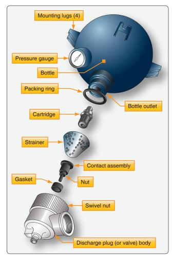
Figure 9-19. Components of fire extinguisher container.
