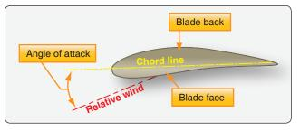
Figure 7-2. Cross-sectional area of a propeller blade airfoil.
