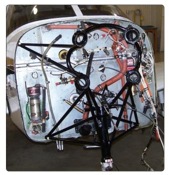
Figure 8-16. Engine mounting ring.
