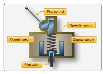
Figure 7-19. On-speed condition.
