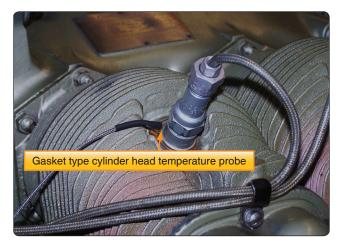
Figure 6-59. Gasket type CHT probe.
