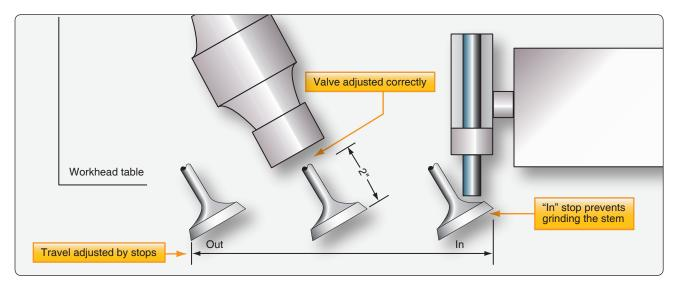
Figure 10-24. Valve installed in grinding machine.
