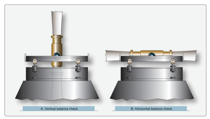
Figure 7-38. Positions of two-bladed propeller during a balance check.
