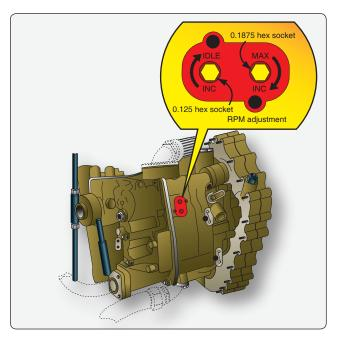
Figure 8-14. Typical fuel control adjustments.
