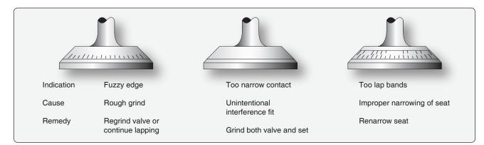
Figure 10-29. Incorrectly lapped valves.
