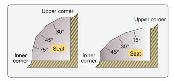
Figure 10-22. Valve seat angles.
