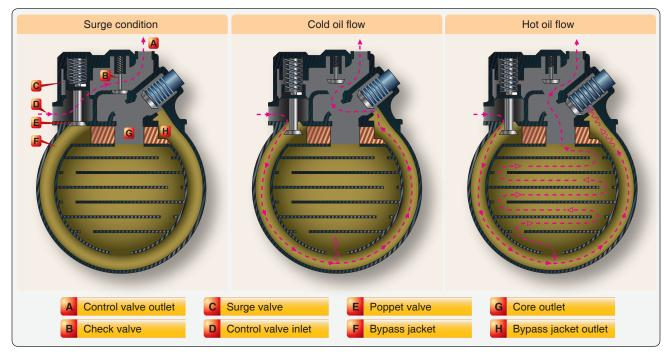
Figure 6-12. Control valve with surge protection.
