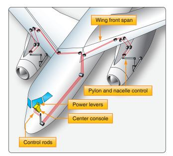
Figure 8-13. Power lever control system.
