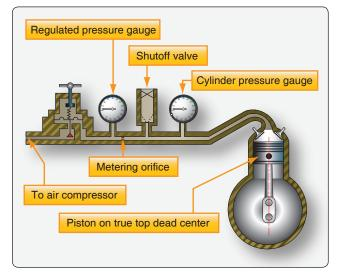
Figure 10-53. Differential compression tester diagrams.
