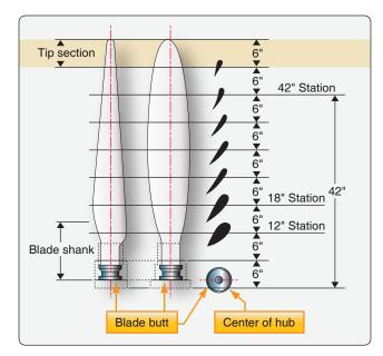
Figure 7-6. Typical propeller blade elements.
