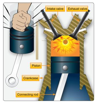
Figure 10-43. *Detonation within a cylinder*.
