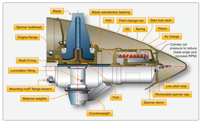
Figure 7-25. Constant-speed feathering propeller.
