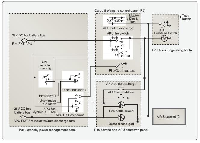
Figure 9-29. APU fire extinguishing circuit.
