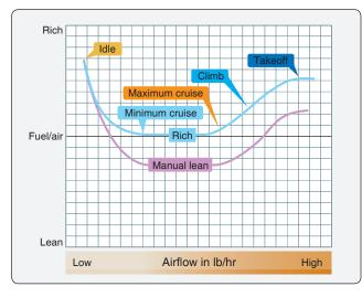
**Figure 10-47.** *Typical fuel-air mixture curve for a float-type carburetor.*
