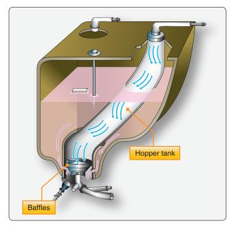
Figure 6-5. Oil tank with hopper.
