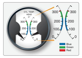
Figure 10-39. Cylinder head temperature gauge.
