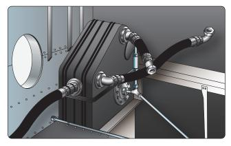
Figure 6-20. Disconnect oil lines.
