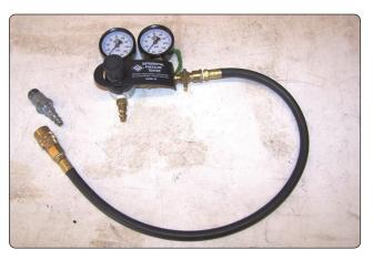
Figure 10-54. Compression tester and adapter.
