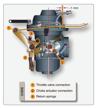
Figure 11-30. Bowden cable routing.
