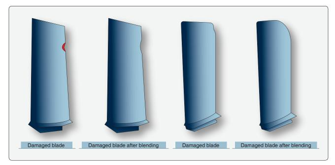
Figure 10-58. Examples of repairs to damaged blades.
