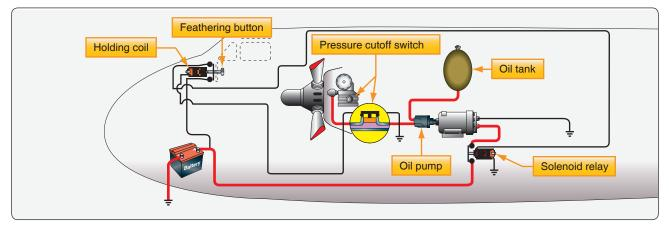
Figure 7-57. Typical feathering installation.
