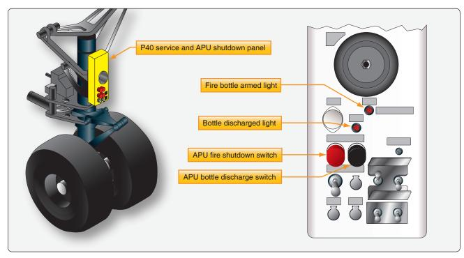
Figure 9-28. P40 service and APU shutdown panel.
