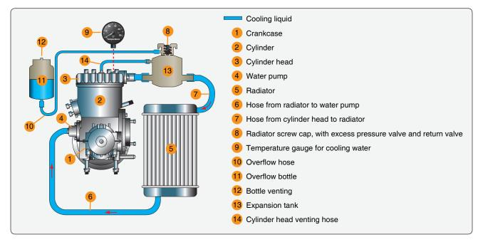
Figure 11-4. Rotax 582 cooling system.
