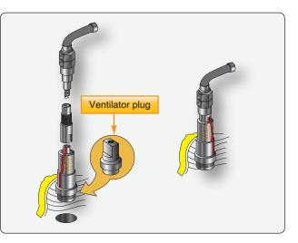
Figure 8-20. Ignition harness lead support installation.
