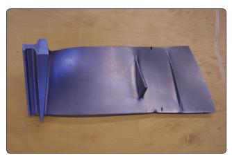
Figure 10-59. Fan blade damage.
