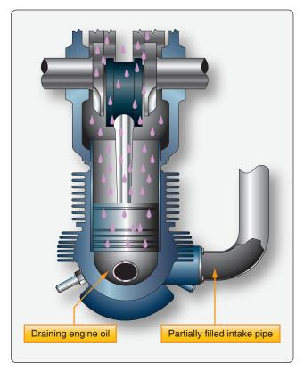
Figure 10-41. *Initial step in developing a hydraulic lock.*
