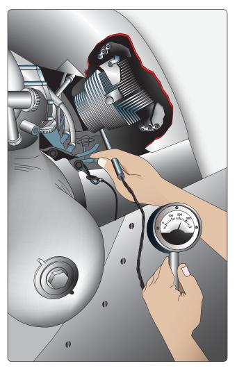
Figure 10-55. Cold cylinder indicator.
