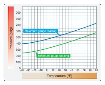
Figure 9-18. Fire extinguisher container pressure-temperature chart.
