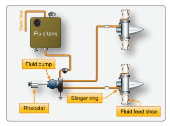
Figure 7-27. Typical propeller fluid anti-icing system.
