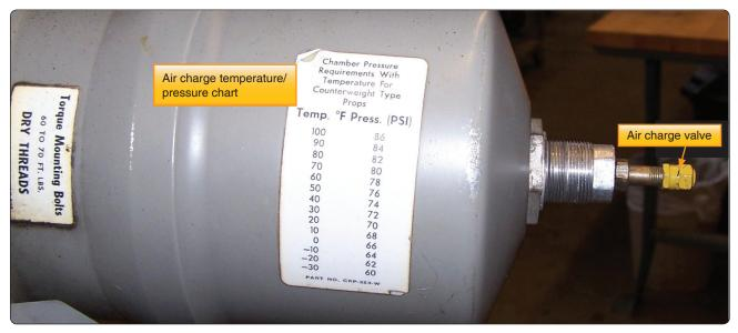
Figure 7-41. Servicing air charge in propeller.
