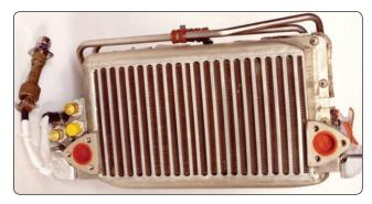
Figure 6-42. Air oil cooler.
