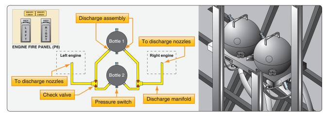
Figure 9-24. Location of fire extinguishing bottles.
