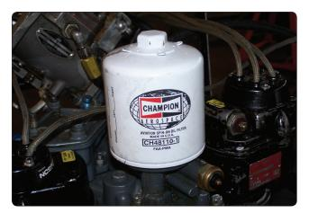
Figure 6-8. Full flow spin-on filter.
