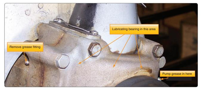
Figure 7-42. Lubricating propeller bearings.
