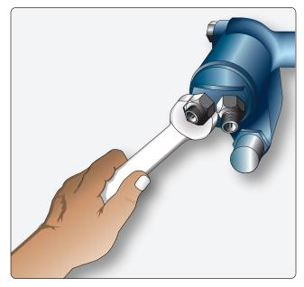
Figure 6-25. *Removing oil temperature bulb.*
