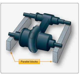
Figure 10-13. Checking connecting rod squareness.
