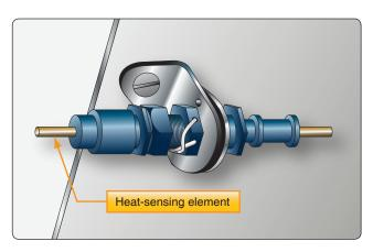
Figure 9-15. Connector joint fitting attached to the structure.
